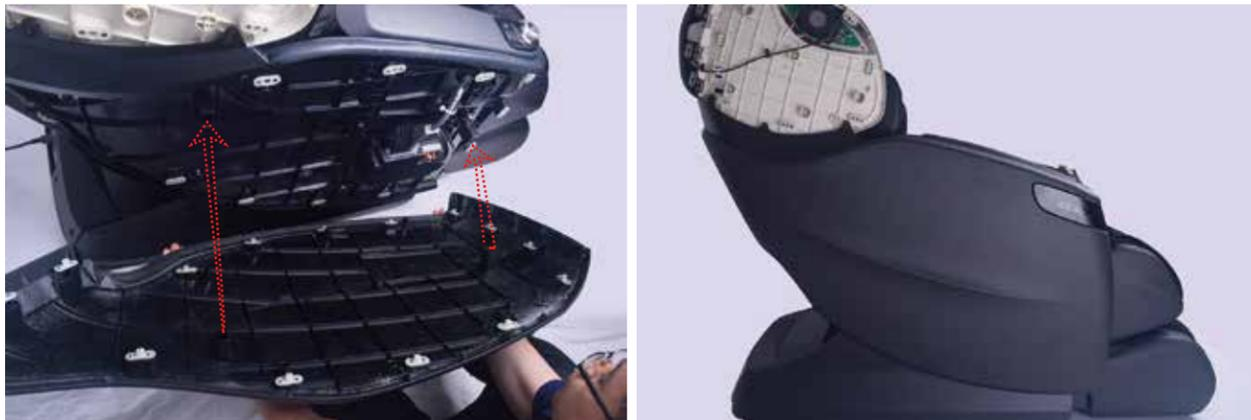
**15 Attach the speaker covers.** These are also attached by snap joints. Attach the side covers first, then the decoration strip on the top.
